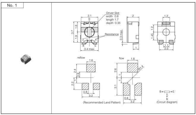
Note: Mounting not possible after trimming knob has been rotated.
